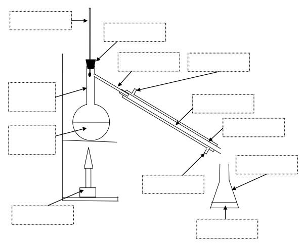
5. Add labels to the parts of the distillation apparatus: DISTILLATE, STOPPER, THERMOMETER, DELIVERY TUBE, CONDENSER, ROUND BOTTOM FLASK, BURNER, MIXTURE, COLD WATER, WATER FROM THE TAP, WATER TO THE SINK, COLLECTING FLASK.
