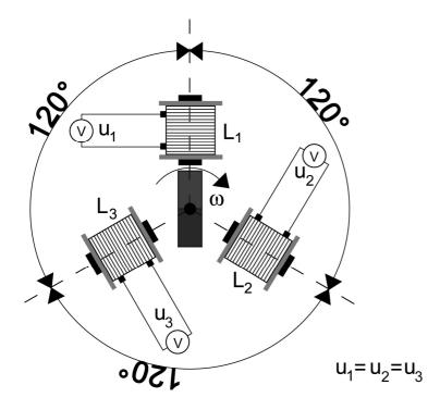
We supply mechanical energy to rotate an (electro)magnet – *rotor* – inside a system of coils – *stator*. For the coils the magnetic field changes and voltage is induced according to the graph below.
