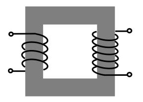
A transformer is a device used to ...... of alternating voltage and current. It consists of two coils and a common core made of ..... = laminations. The alternating current passes the primary coil and it creates a ...... magnetic field around it. This field is ..... by the iron core and ..... with the secondary coil. Due to electromagnetic induction, voltage is ...... on the secondary coil.
