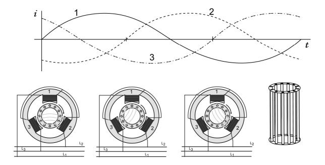
**Note:** We can use a magnet rotating inside the set of coils instead the squirrel cage, so that there is no delay. This motor is in general less suitable for powerful machines.
