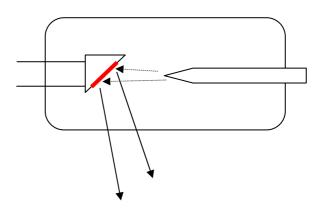
principle – electrons (1) produced by thermionic emission on cathode (2) are accelerated towards anode (3); as they hit the target (4) about 0.5% of their E<sub>k</sub> is converted into the X-rays (5)
