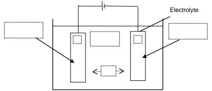
2. Label the diagram above with the following: pure Cu, impure Cu, +, -,  $CuSO_4$ ,  $Cu^{2+}$  and choose the correct direction of the arrow.
